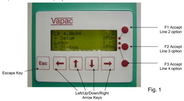
Figure 1 above shows the Alphanumeric keypad and display. This gives four lines of information, with each line having a maximum of twenty characters. The Arrow keys are used to navigate through the menus and the round buttons, on the right hand side, are used to action the associated options:
