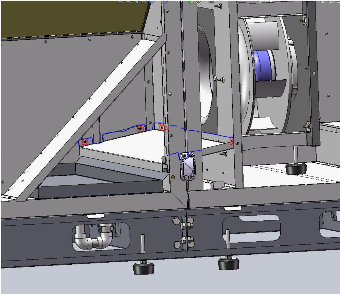
5. Connect unit sections electrically. Connect cable connectors. According to the markings
