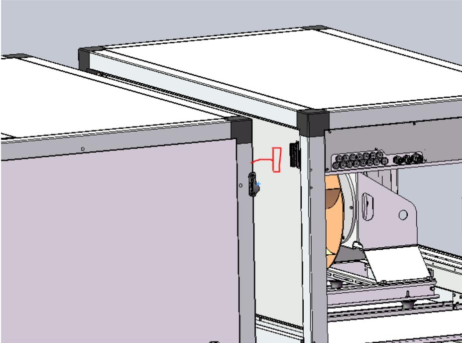
3. The sections are pushed together side by side, and connected with bolts
