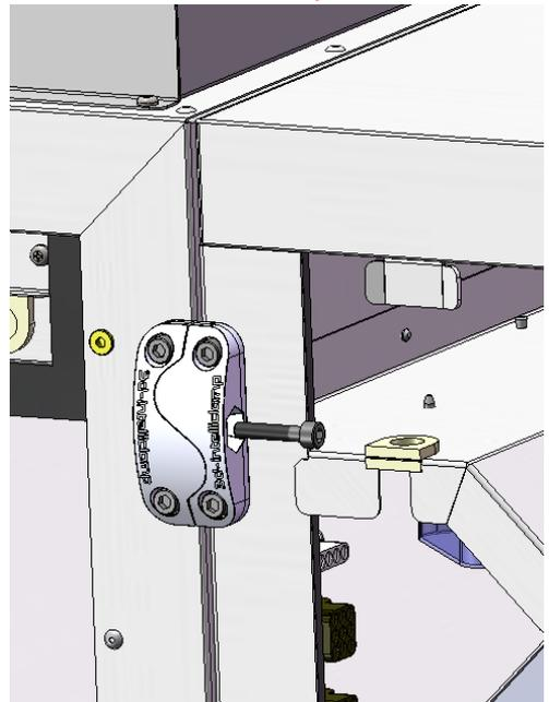
4. Screw condensate drain detail. The blue marked places grease with sealant.
