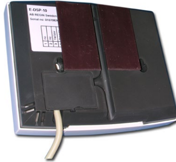
Figure 1. The cable is led through the outlet
