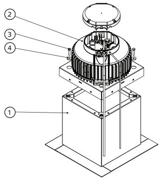
■ Fasten the roof fan (2) with screws and washers (3) and (4) on the roof socket (1)
