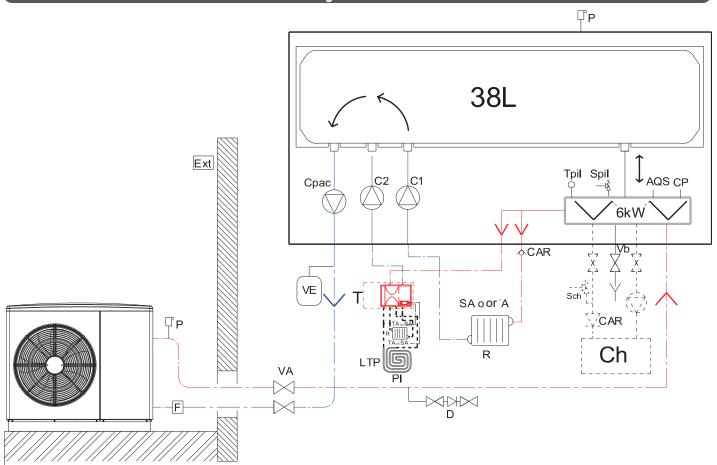
**AQS** Aquastat CAR Non-return valve Ch Boiler back-up (optional) CP Pressure sensor Cpac: HP circulator C1 Circuit 1 circulator C2 Circuit 2 circulator D Filling valve Ext Outside sensor F Filter Valve LTP OPT - Overheat protection thermostat
