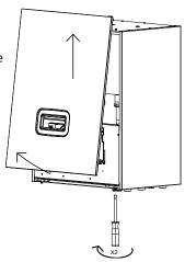
2- Pull the base of the front panel forwards, and lift the panel to unhook the pegs located at the top of the **Pilot**.
