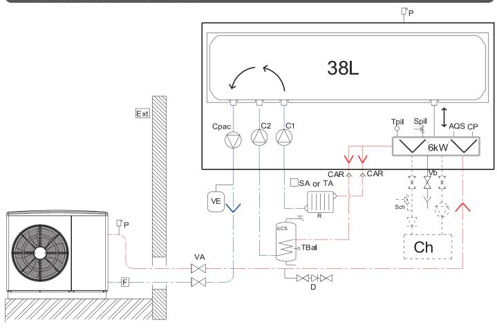
AQS Aquastat CAR Non-return valve Ch Boiler back-up (optional) CP Pressure sensor Cpac: HP circulator C1 Circuit 1 circulator **C2** Circuit 2 circulator D Filling valve **ECS** DHW tank Ext Outside sensor Filter Valve
