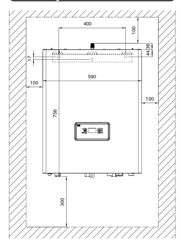
Place and fix the mounting bracket on the wall first.
