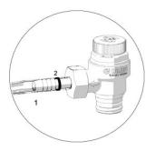
The EPDM pipe must be pushed to the end of the safety valve barb tip and held with a hose clamp.
