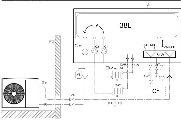
AQS Aquastat CAR Non-return valve Ch Boiler back-up (optional) СP Pressure sensor Cpac: HP circulator C1 Circuit 1 circulator C2 Circuit 2 circulator D Filling valve Ext Outside sensor Filter Valve
