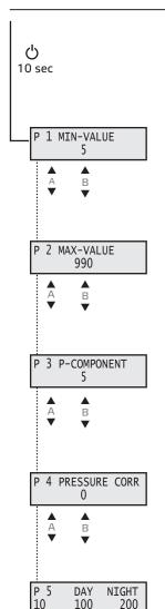
You move to the parameter settings menu menu P by pressing the ON/OFF button, which must be held down for approx. 10 seconds.
