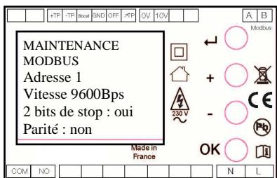
To access these parameters, press the OK button for 5s and follow the tree explained in chapter V.1.
