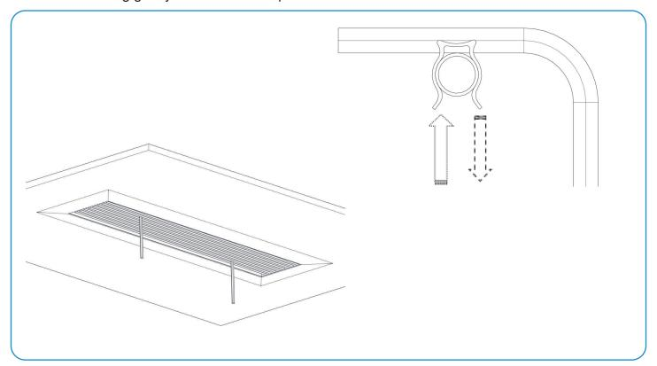
5.1.2- Once the finned core has been completely released from the grille frame, hold it, remove the anti-fall safety chord and remove the core.
