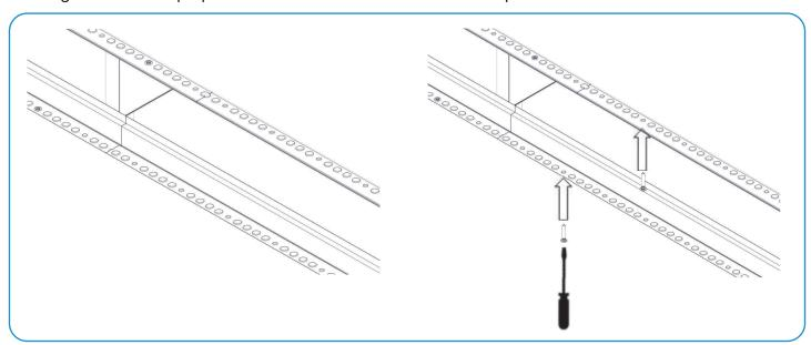
4.5- Once the grille has been fixed with the screws, plaster over the all the holes drilled along the entire row and finish with a fine paste.
