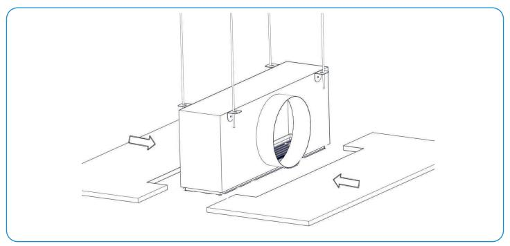
4.1B.4- Once the boards are installed, insert and fix the grille using at least 4 plasterboard screws in the smaller Ø4mm holes drilled on the grille lid for the purpose. The distance between each screw pair should not exceed 250 mm.
