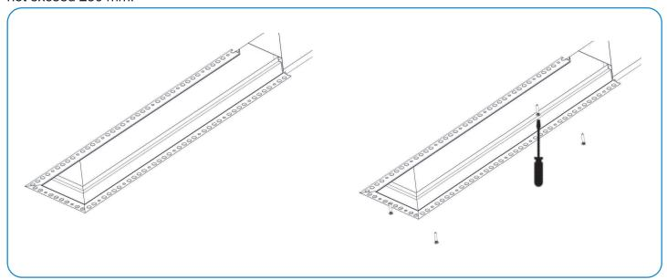
Where the plenum boxes are fitted independently of the grille, it is not necessary to fix them together. The plenum box should be fixed to the ceiling slab and the grille to the plasterboard. This allows supply and return air rows to be designed according to requirements of the project.
