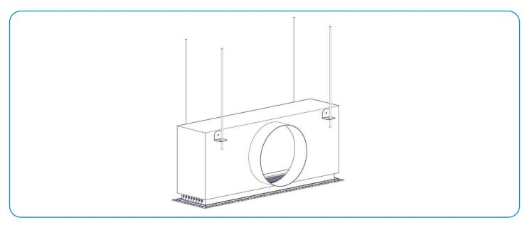
3.1- Fix the plenum box using threaded rods. Use the threaded rods to adjust the height of the unit so that the lower edge of the grille is level with the underside of the ceiling.
