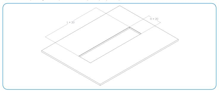
2.2- The distance between the grille and the ceiling support frame should not exceed 150 mm.
