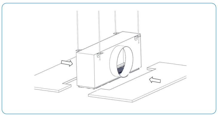
3.4- Fix the grille using at least 4 plasterboard screws in the smaller Ø4mm holes drilled on the grille lid for this purpose. The distance between each screw pair should not exceed 250mm.
