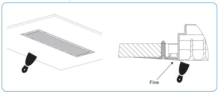
4.6- Once the entire row has been installed, install the cores of each section. Offer up the core to the frame and once the tubes of the fin block are aligned with the pressure clips, push up until the tubes clips in.
