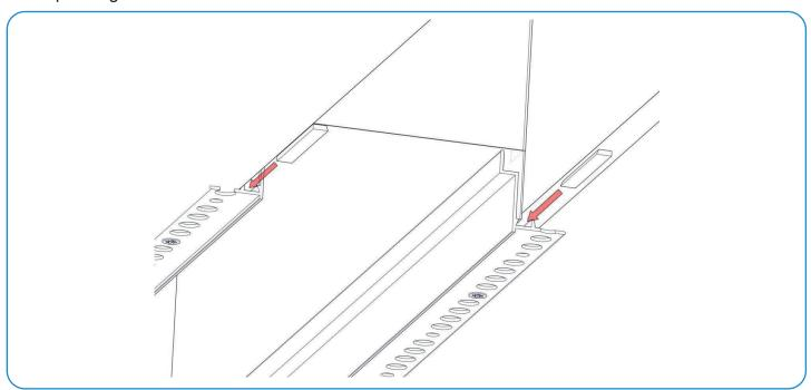
4.3- Set the grille at the height of the plasterboard and adjust it horizontally so that the alignment bands to build the rows fit into the rail of the corresponding frame.
