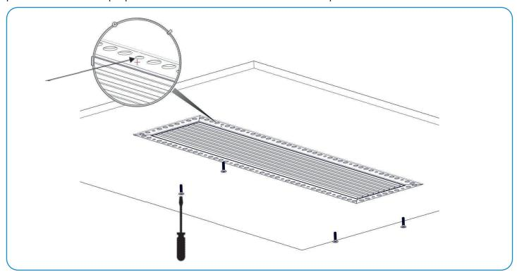
2.5- Once the grille is fixed with the screws, plaster over the holes in the perimeter lid of the grille and finish with a fine paste.
