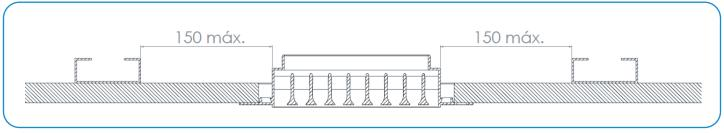
2.3- Position the grille in the opening in the plasterboard and raise it until the perimeter lid of the grille touches the ceiling.
