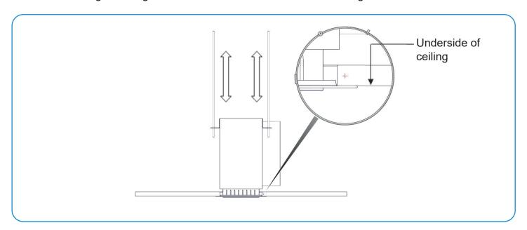
3.2- The distance between the grille and the ceiling support frame should not exceed 150 mm.
