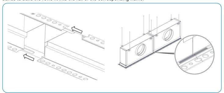
4.4- Fix the newly installed section using at least 4 plasterboard screws in the smaller Ø4mm holes drilled on the grille lid for this purpose The distance between each screw pair should not exceed 250 mm.
