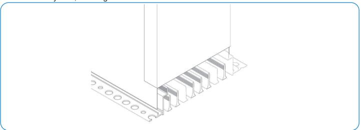
4.1A.2- Install the plenum box + grille assembly according to the instructions in part 3 above. Make sure the plenum boxes at the start/end of the row are installed first, followed by the intermediate plenum boxes.
