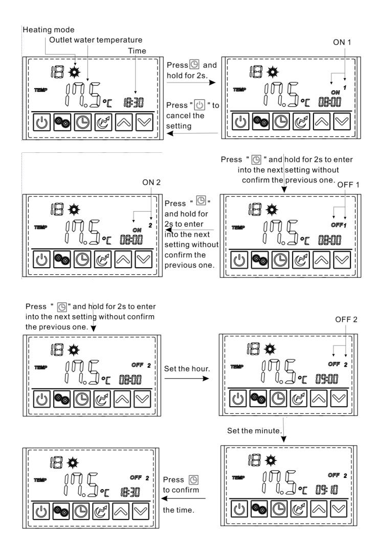
Example: Running period 1: 8:00~10:00; Running period 2: 16:30~20:00. ON 1 Outlet water temperature Current time Press " #:30 and hold for 2s Confirm the time after setting. OFF 1 ON 2 **1**□ **\*** Confirm the time after setting. Confirm the time after setting. Press" "to confirm OFF 2 Successful setting Press "" to cancel
