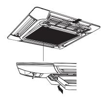
5. Close the intake grille and push the intake grille's hooks outward.
