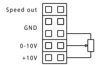
Connection with enclosed potentiometer
