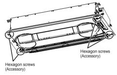
• Ensure that there is no gap between the indoor unit and the grille at these four locations.
