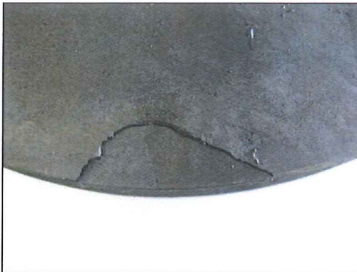
Crack in the outer cover
