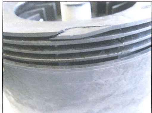
Crack in the outer cover
