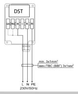
Hi / N / Pe - 3rd fan speed Med. / N / Pe - 2nd fan speed Low / N / Pe - 1st fan speed
