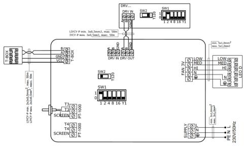
T-BOX - S-TOUCH controller with touch screen connection
