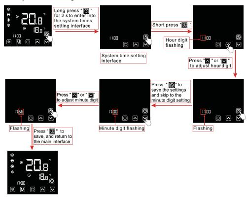
Notes: Under the clock setting interface, if there is no operation for 20 s, the system will automatically memorize use's settings, and return to the main interface; if short press under the main interface, if short press under the changes will not be saved and return to the main interface.
