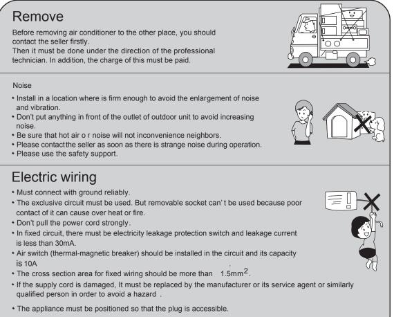
• The appliance should be installed in accordance with national wiring regulations.
