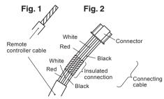
Connect the remote controller cable to the connecting cable, and insert it to the connector.
