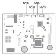
This air conditioner can be connected with the following optional type. For details on how to install optional parts, refer to the installation manual included in each item
