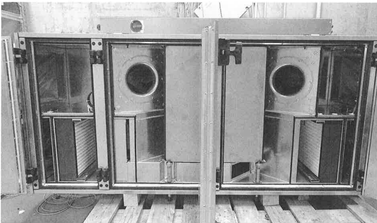
Fig. 2 Internal layout of the air handling unit
