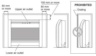
When embedding the indoor unit in a wall, restrict the movement of the horizontal vane for the upper air outlet so that it only operates horizontally. If this setting is not performed, heat will build up in the wall and the room will not be cooled or warmed properly.
