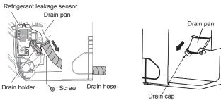
NOTE: When attaching/removing the drain holder and drain hose on the refrigerant leakage sensor side, be very careful not to give a shock to the sensor.
