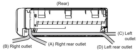
Example: In the case of Right outlet (Although the figure in the case of Left outlet is omitted, the same shall apply.)
