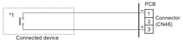
\*1: The switch can be used on the following condition: DC 12 V to 24 V, 1 mA to 15 mA.
