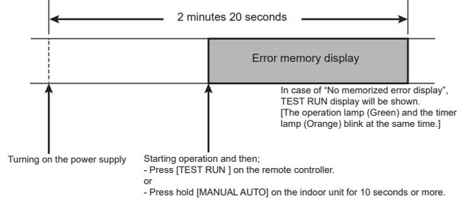
\*: The "3 minutes ST" period lasts 2 minutes and 20 seconds after turning on the power supply.
