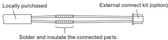
4.1.2. Installing the External input/output PCB
