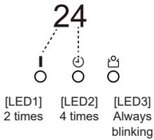
The first and second digits of the error code are indicated by the number of times the lamp blinks.
