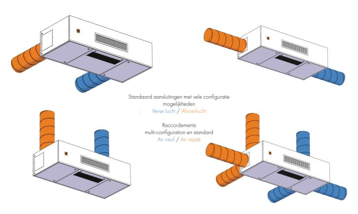
The Eversky is **only** available in a **right** execution, viewed from the top of the device, following the direction of the airflow. **This unit is supplied as standard with the possibility to easily change rear connections to side or top connections on site!**
