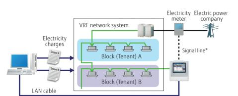
\*: Electricity meter (1unit) can be connected to external input connector of the TPC unit.
