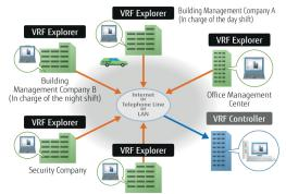
1 VRF Controller can be monitored from any number of VRF Explorers (Up to 5 connections simultaneously).
